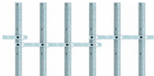
■ FIGURE 12: FAST-FIX NOGGING® INSTALLATION
