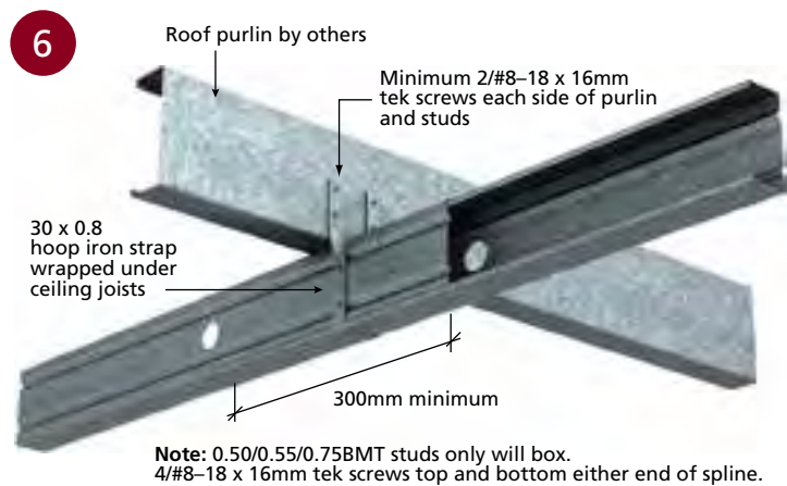
■ SUSPENSION JOINT TYPE 1
